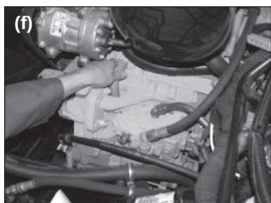
Inspecting the coolant hoses.
