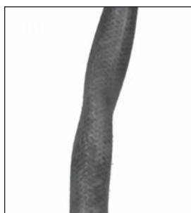
Partly collapsed inlet line shown.
