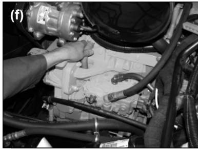
Inspecting the coolant hoses.
